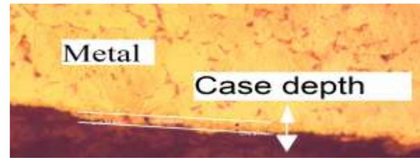
**Figure 1: Micrograph and case depth of carburized steel according to (Taguchi) array (1000x).**
