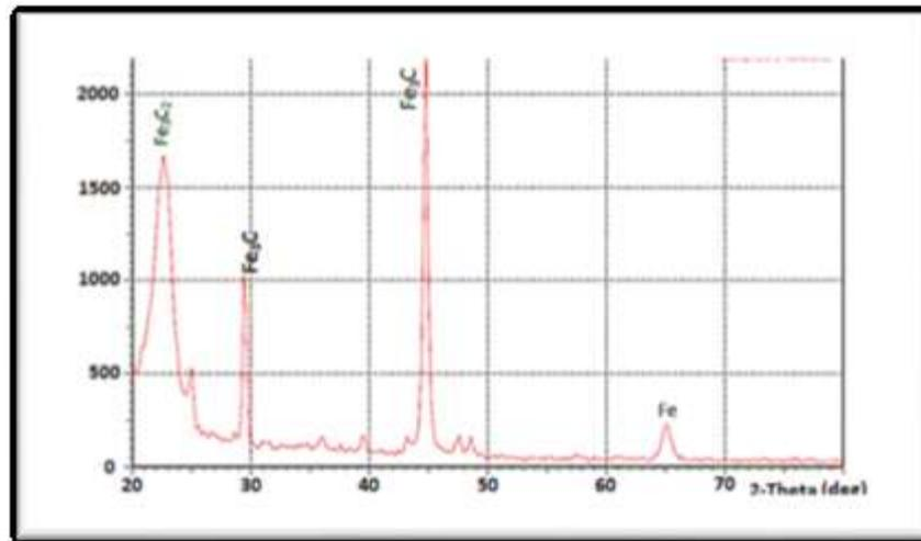
**Figure 2: Diffraction spectra of steel carburized at optimum conditions.**
