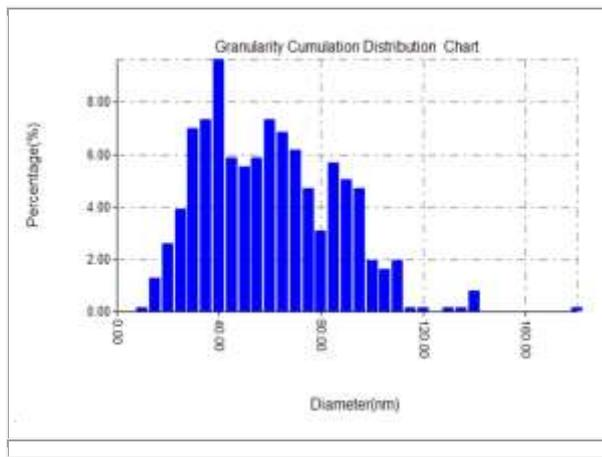
Figure 2: AFM Test of Nano- $\text{Al}_2\text{O}_3$  Particles.
