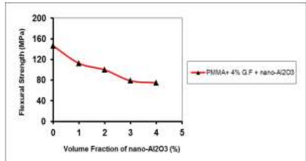
Figure 10: Flexural Strength of PMMA Hybrid Laminated Composite as Function of (Nano-Al<sub>2</sub>O<sub>3</sub>) Particles (Vol. %) in Composite.
