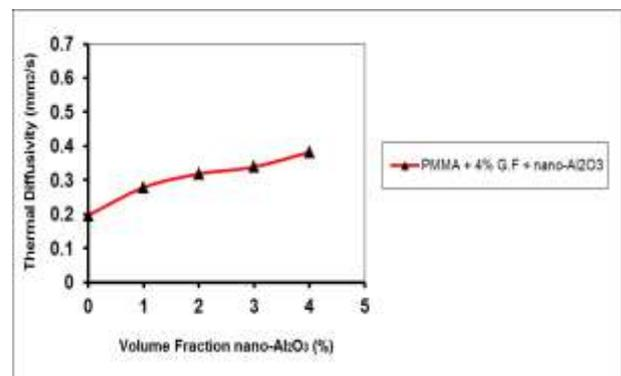
Figure 17: Thermal Diffusivity of PMMA Hybrid Laminated Composite as Function of (Nano-Al<sub>2</sub>O<sub>3</sub>) Particles (Vol. %) in Composite.
