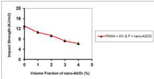
Figure 8: Impact Strength of PMMA Hybrid Laminated Composite as Function of (Nano-Al<sub>2</sub>O<sub>3</sub>) Particles (Vol. %) in Composite.
