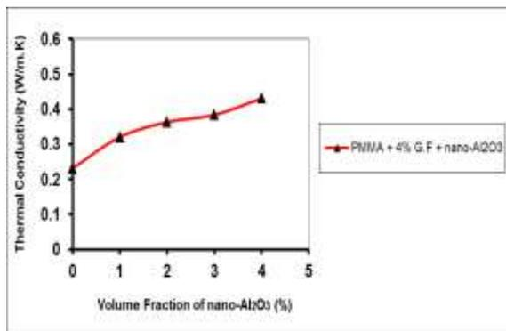
Figure 16: Thermal Conductivity of PMMA Hybrid Laminated Composite as Function of (Nano-Al<sub>2</sub>O<sub>3</sub>) Particles (Vol. %) in Composite.
