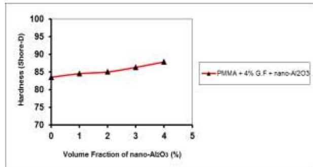
Figure 13: Hardness of PMMA Hybrid Laminated Composite as Function of (Nano- $\text{Al}_2\text{O}_3$ ) Particles (Vol. %) in Composite.
