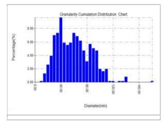
Figure 2: AFM Test of Nano-Al<sub>2</sub>O<sub>3</sub> Particles.
