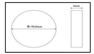
Figure 12: Schematic Specimen for Standard Specimen of Hardness Test.
