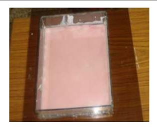
Figure 3: Casting of Composite Specimens in Glass Mould.
