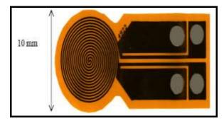
Figure 14: Hot Disk Sensor
