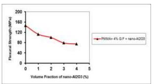
Figure 10: Flexural Strength of PMMA Hybrid Laminated Composite as Function of (Nano-Al<sub>2</sub>O<sub>3</sub>) Particles (Vol. %) in Composite.
