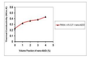
Figure 16: Thermal Conductivity of PMMA Hybrid Laminated Composite as Function of (Nano-Al<sub>2</sub>O<sub>3</sub>) Particles (Vol. %) in Composite.
