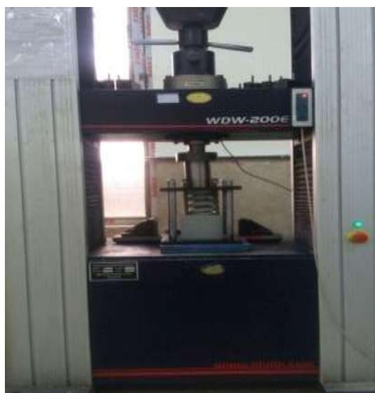
**Figure 3A: The deep drawing tools mounted in the testing machine.**
