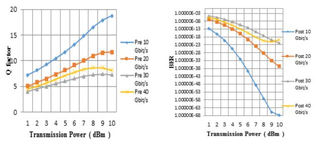
Figure 3: Comparison of transmission power vs Qfactor influence of various Bit rates for pre- scheme BER influence of various Bit rates for post- scheme
