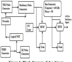
Figure 1: Block diagram of duo-binary transmitter
