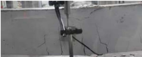
Figure 6: concrete crushing in SL beam
