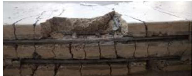
Figure 13: debonding of CFRP bars
