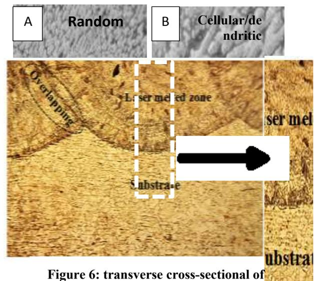
Figure 6: transverse cross-sectional of microstructure after LSM
