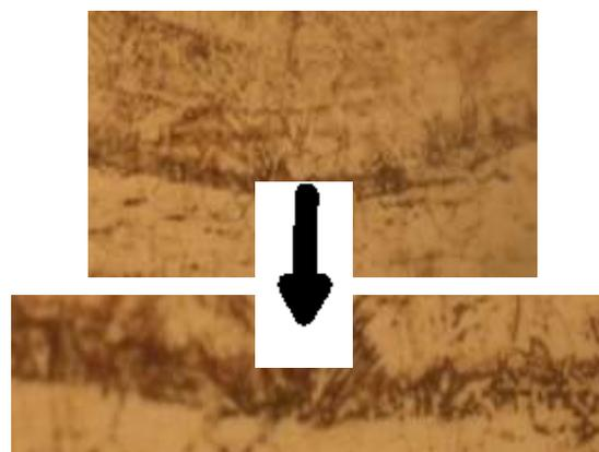
Figure 8: interface zone between melted and substrate
