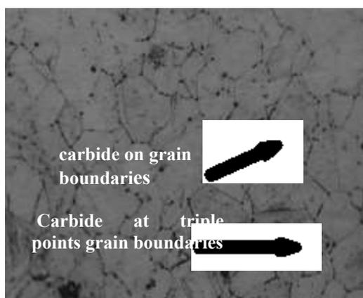
Figure 5: sample after heat treated (aging) at 800°C for two hours
