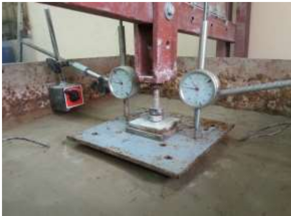
Plate 6: Loading assembly of the test.
