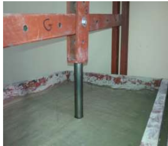
Plate 4: Installation of the model pile in the clay
