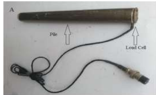
Plate 2: Instrumented model pile with load cell..
