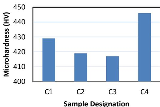
Figure 5: Microhardness of enameled cast iron
