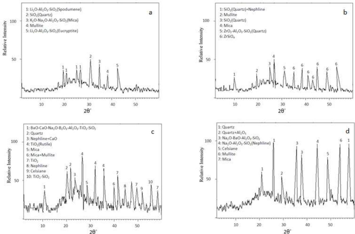
Figure 4: X-ray diffraction of cast iron enamel (a) enamel containing  $\text{Li}_2\text{O}$  (b) enamel containing  $\text{ZrO}_2$  (c) enamel containing  $\text{TiO}_2$  (d) enamel containing  $\text{CaO}\cdot\text{Al}_2\text{O}_3\cdot 2\text{SiO}_2$
