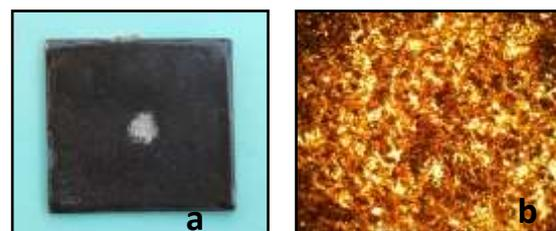
Figure 7: Photograph and microstructure of the peeled surface of coating by the adhesion test
