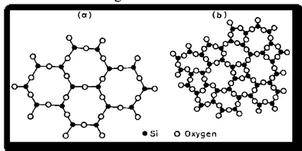
Figure 1: a- Crystalline structure (regular). b- glassy structure (irregular) [9]
