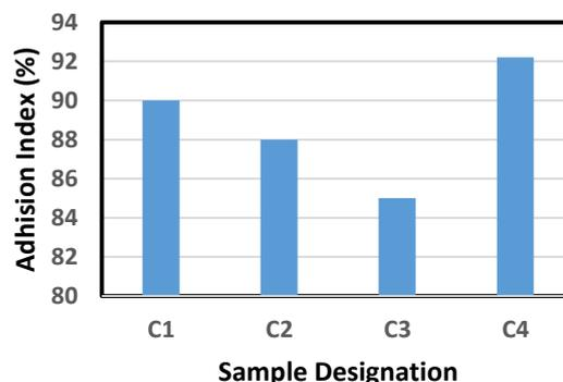
Figure 6: Adhesion index (%) of enameled cast iron
