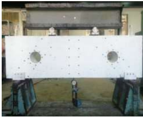
Plate 4: Test setup for deep beam specimen
