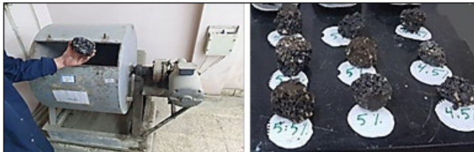
Figure 5: Samples during and after (Cantabro) Abrasion Loss Resistance Test
