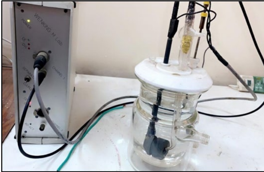
Figure 2: Figure 2: The cyclic potential dynamic polarization test device
