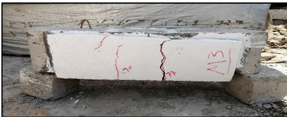
Figure 10: Cracks in reinforced concrete beam strengthened with type 3 Ferro-cement layer
