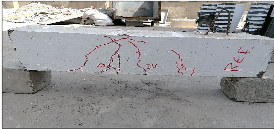
Figure 7: Failure Cracks in the reference beam
