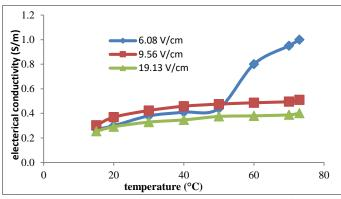
Figure (3): The effect of electrical conductivity on the temperature of pasteurized milk at different voltage gradients.
