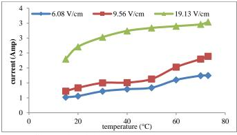
Figure (4): Temperature profile as electrical current passing through the milk at different voltage gradients.
