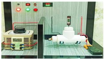
Figure (2): batch type ohmic heating equipment
