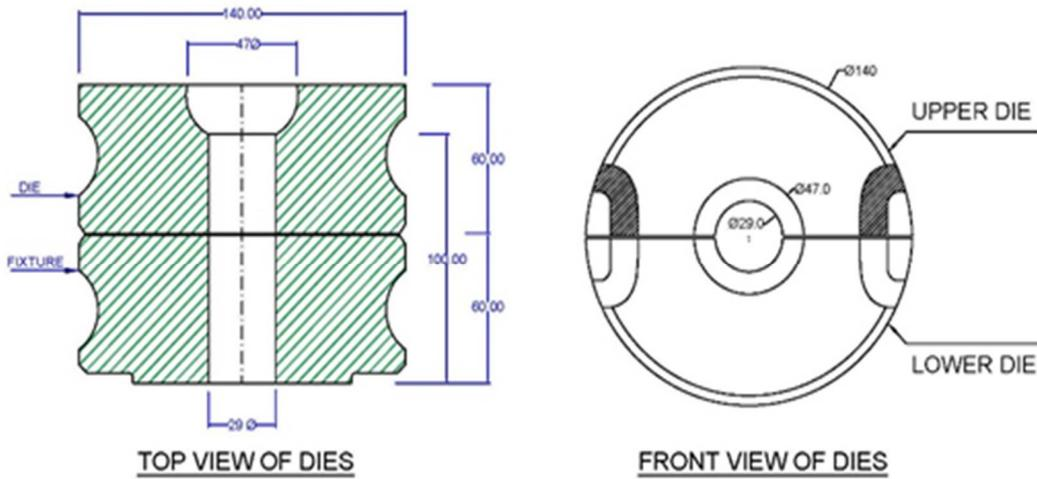
**Figure 3:** Dimensions of upper and lower die with fixture Compare shapes
