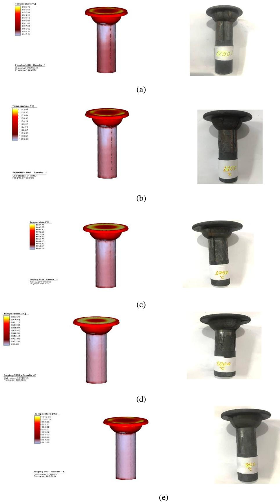
Figure 4: Experiment Result and Analysis at (a) 1150 °C (b) 1100 °C (c) 1050 °C (d) 1000 °C (e) 950 °C
