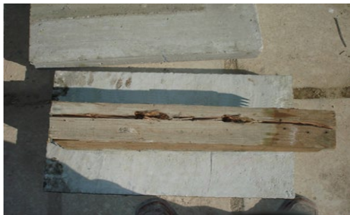
Figure 7: The longitudinal flaw in the timber beam after the failure of the push-out specimen
