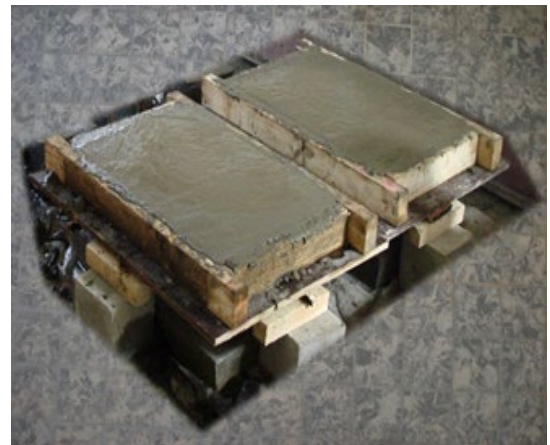
Figure 3: The casting of the second slab for push-out specimens
