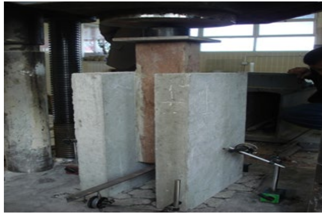
Figure 4: Push-out test arrangement
