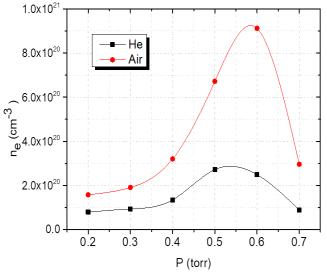
Fig. (6) shows the range of change of the electron density with the pressures that were chosen for dry air and helium gas at the distance between the electrodes 12 cm and constant power of 0.6 watt.
