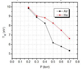
Fig.(5) shows the variation of electron temperature with the gas pressure at an inter-electrode distance is 12 cm and the power is constant 0.6 watt for dry air and helium gases.
