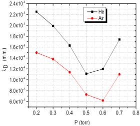
Fig. (8) The change in Debye length with the change of pressure for dry air and helium as working gases at interelectrodes distance equal 12 cm and constant discharge power of 0.6 watt.
