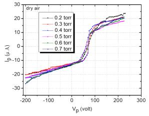
Fig. (3) The I-V characteristics of the double probe for dry air at the inter-electrodes distance is 12 cm and a constant power of 0.6 watt.
