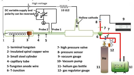
Fig. (1) Schematic diagram of the capillary dc glow discharge system
