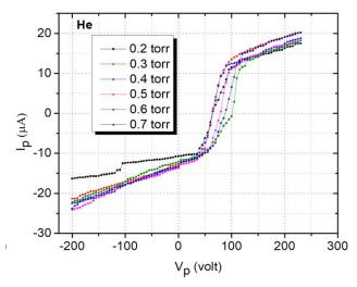
Fig. (4) The I-V characteristics of the double probe for Helium at the inter-electrodes distance is 12 cm and constant power of 0.6 watt.
