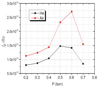
Fig. (9) The change in plasma frequency as a function pressure for dry air and helium as working gases at interelectrodes distance equal 12 cm and constant discharge power of 0.6 watt.
