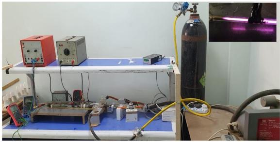
Fig. (2) Photograph of the complete system of continuous capillary glow discharge.
