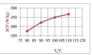
Figure 4 Temperature of bed hot water effect on SCP Tc=30°C, Tch= 20°C, t half-cycle = 320 s
