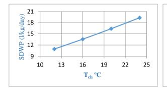
Figure 6 Effect of evaporator water temperature on SDWP Tc=30°C, Tb= 90°C, t half-cycle = 320 s
