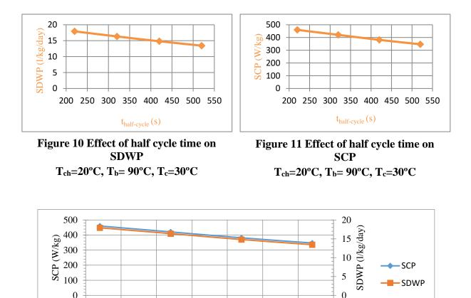
Figure 12 SDWP & SCP of 2-beds cycle utilize silica-gel/water pair. Tb=90°C, Tc=30°C, Tch=20°C
