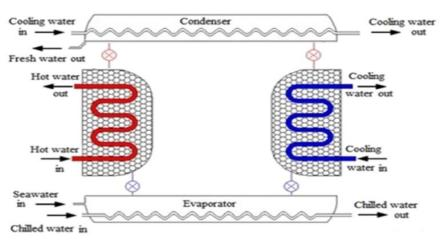
Figure 1 Schematic diagram of AD system[1].
