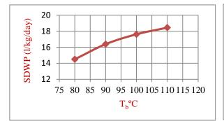
Figure 3 Temperature of bed hot water effect on SDWP Tc=30°C, Tch= 20°C, t half-cycle = 320 s
