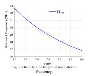
The dimensions of the resonators in generalized Chebyshev filter are calculated by amount of deviation in the resonant frequency of each resonator  $f_{ox}$  from the center frequency of the filter  $f_o$  depending on the coupling coefficient of each element with itself  $M_{ii}$  in the coupling matrix of the filter[10].
