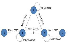
Fig. 9 Coronal shape of the coupling coefficients of a third-order generalized Chebyshev filter with (TZ) below the passband.
