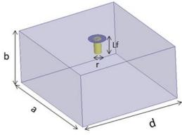
Fig. 3 Coaxial probe feeder.
