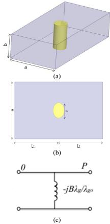
Fig. 4 Inductive coupling between two resonators using a post (a) 3D view (b) top view (c) equivalent circuit.
