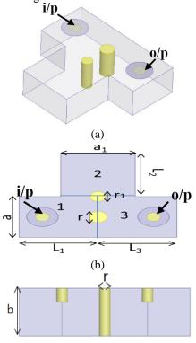
(c) Fig. 12 A third-order filter with a passing zero above the passband (a) 3D view (b) top view (c) side view.
