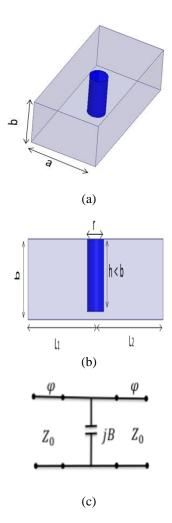
Fig. 5 Capacitive coupling between two resonators using a post (a)3D view (b) top view (c) equivalent circuit.
