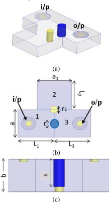
Fig. (8) A third-order filter with a TZ below the passband 3D view (b) top view (c) side view.
