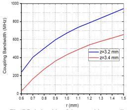
Fig. 7 Relationship of the capacitive coupling bandwidth with the diameter of the post at varing depth inside the resonator.
