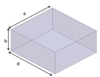
Fig. 1 Rectangular waveguide cavity resonator.
