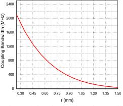
Fig. 6 Relationship of the inductive coupling bandwidth of a single post against the diameter of the post.
