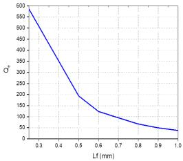
Fig. 3 Relationship of the length of the feed probe to the external coupling.
