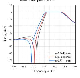
Fig. 11 Insertion loss response with controlling (TZ) position below the passband.
