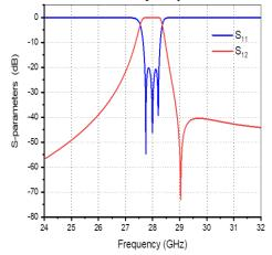
Fig. 14 S-parameters of a third-order generalized Chebyshev type filter with a (TZ) above the passband.
