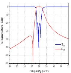
Fig. 10 S-parameters of a third-order generalized Chebyshev BPF with a TZ below the passband.
