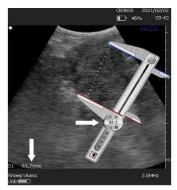
Figure 1: Calibration of the Screen Caliper software through an image of the ultrasonic device with known distances in millimeters.
