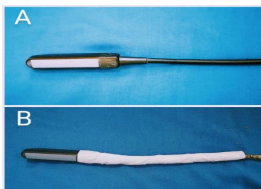
Figure 2: before and after applying the rubber tube to the probe.
