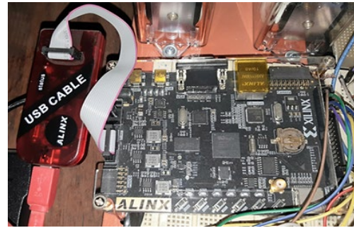
Figure 6: Xilinx Spartan 6 FPGA board (XC6SLX45)
