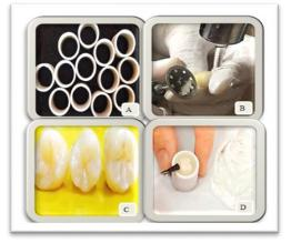
Figure (2): Preparation of Enamel Blocks, (A) Cylindrical Plastic Tubes, (B) Separation Of The Crowns From The Roots, (C) Crowns After Cutting, (D) Cold Cure Acrylic Mold &Varnish Application.
