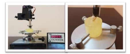
Figure (1): The Clasp on Abutment Fixed on Cycling Machine.
