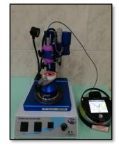
Figure (1): Diode laser handpiece stabilized by milling machine
