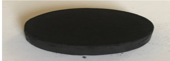
Figure 1: The pellet of \text{Fe}_3\text{O}_4 20 mm diameter and thickness of 6 mm
