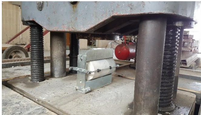
Figure 6. Instrument test to find splitting tensile strength for concrete.
