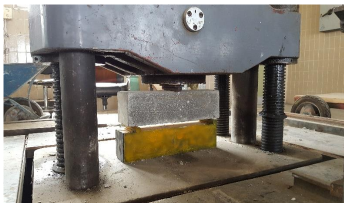
Figure 8. Instrument test to find modulus of rupture.
