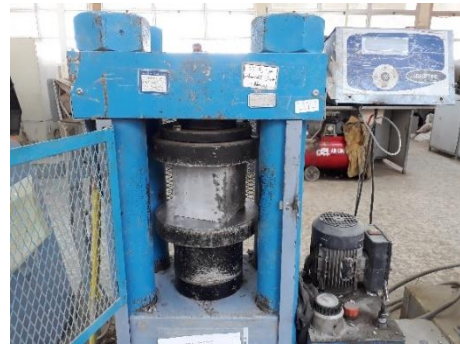
Fig. 2 Compressive strength test machine
