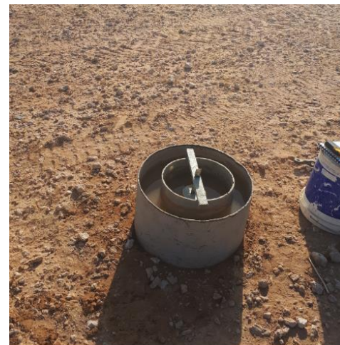
Fig.2. Field infiltration test
