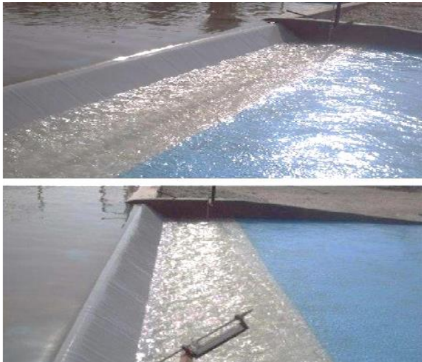
Fig. 3. Physical model of Mandali spillway.
