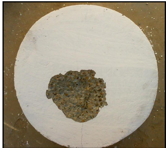
Plate (2) The Mode of Failure of Slabs Specimens under High Velocity Impact
