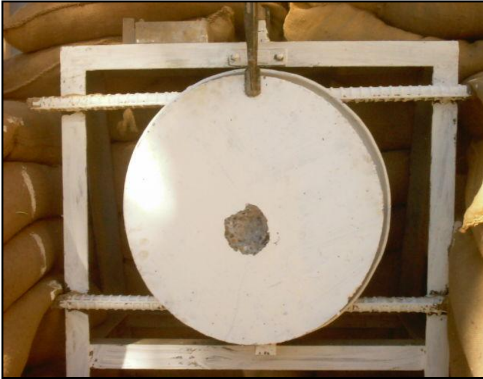
Plate (1) Test Rig Used for High Velocity Impact Test
