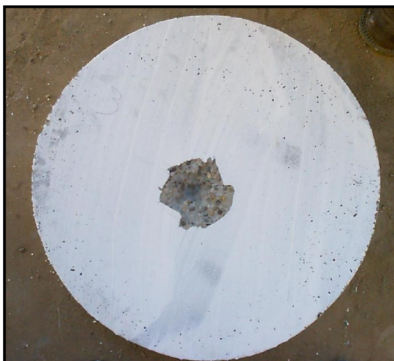
Plate (2) The Mode of Failure of Slabs Specimens under High Velocity Impact
