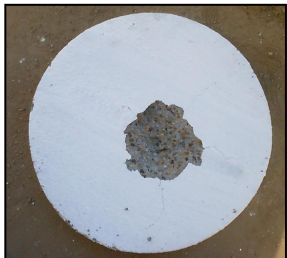
Plate (2) The Mode of Failure of Slabs Specimens under High Velocity Impact
