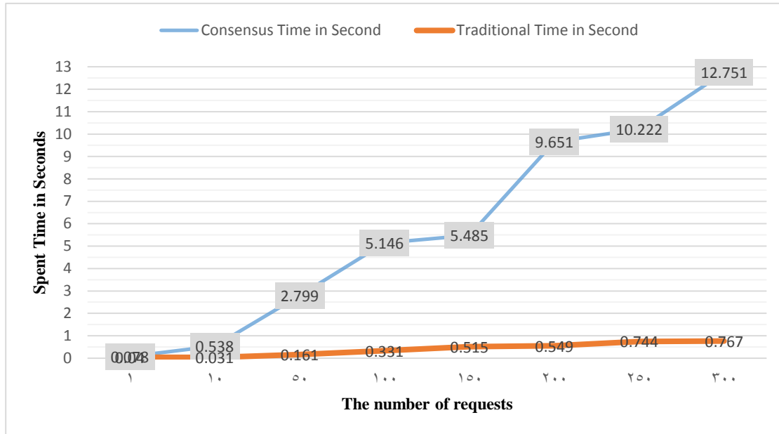
FIG. 5. SPEND TIME OF AUTHORIZATION PROCESSES ON BLOCKCHAIN FOR MULTIPLE REQUESTS
