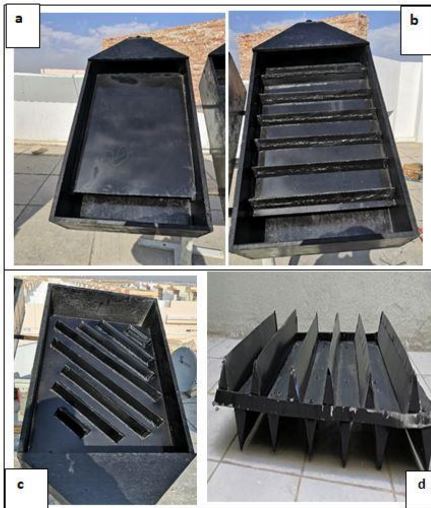
Figure (1): The different configurations of absorber (a: Flat Plate, b: With fins placed perpendicular on airflow , c: With fins placed inclined at an angle 45° , d: With double fins placed perpendicular on airflow )
