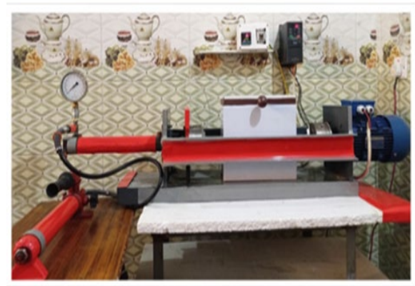
Figure 1: B Actual thermal buckling test device
