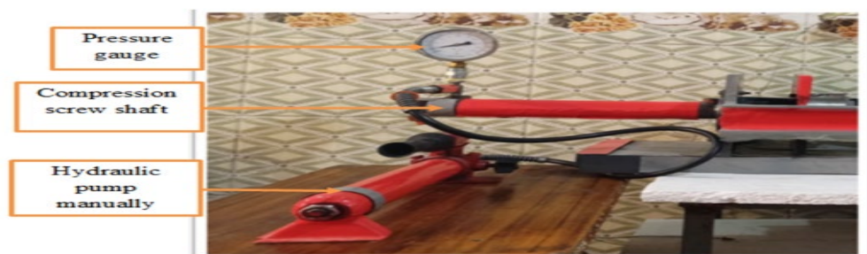
Figure 3: Parts of the compression system
