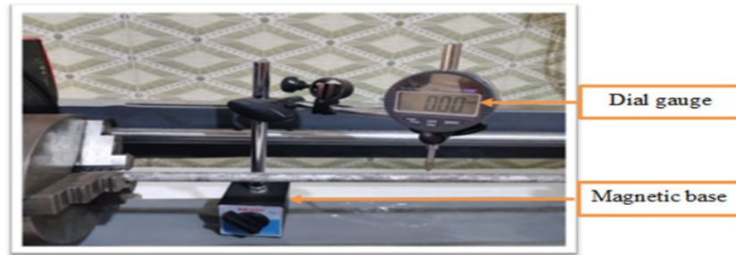
Figure 5: Buckling failure measuring device
