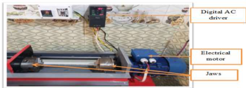
Figure 2: The torsion system
