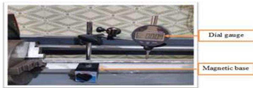
Figure 5: Buckling failure measuring device
