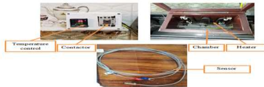
Figure 4: Parts of the electric oven
