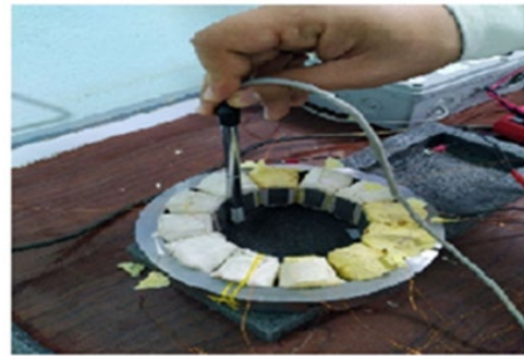
Figure 2: The position sensor for testing the magnetic density for each pole
