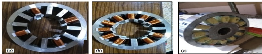
Figure 9: Steps of wrapping the poles
