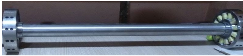
Figure 13: The rotor is made of metal type steel 37-2
