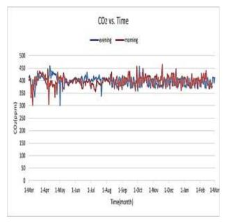
Fig. 3: Rate of CO<sub>2</sub> in Erbil atmosphere during one year at day (red line) and night (blue line). The rate of CO<sub>2</sub> fluctuated between minimum range is (300 ppm) to the maximum value (450 ppm).
