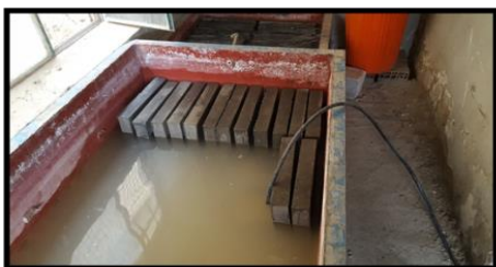
Figure6. Slabs during curing
