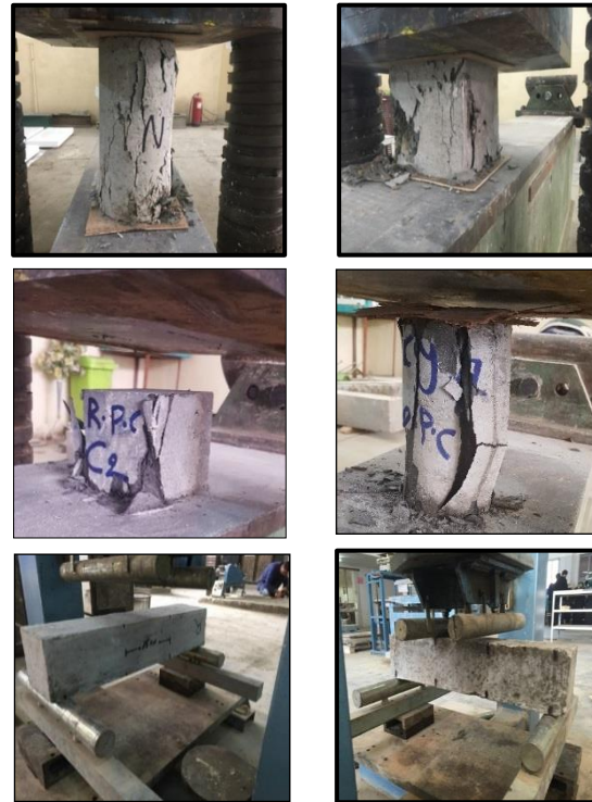
Figure8. the cubes, prisms, and cylinders
