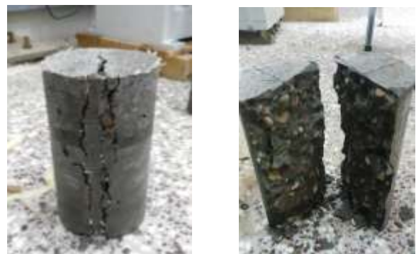
Fibre reinforced specimen Reference specimen
