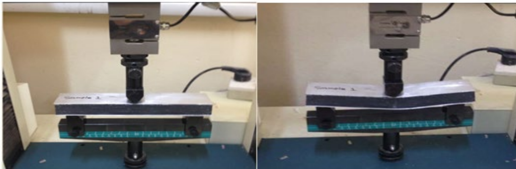
Figure 7: Experimental setup for the FG core sandwich beam
