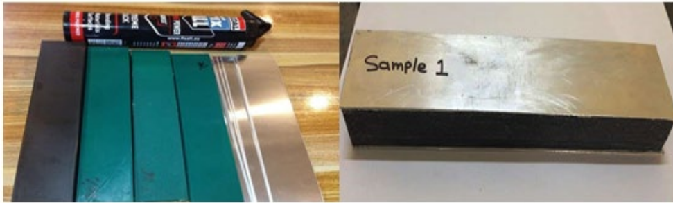
Figure 5: FG sandwich specimens with porous metal core
