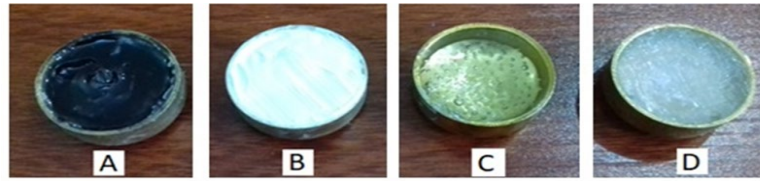
Figure 1: Appearance of different types of adhesives: (A) Epoxy Resins (B) MS Hybrid Polymers (C) Polyvinylester (D) R.T.V Silicon Rubber
