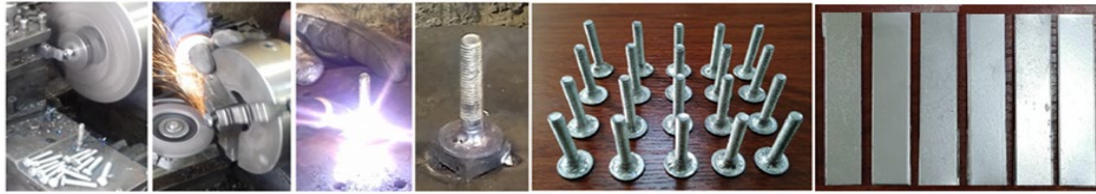
Figure 4: Manufacture and prepare the adherent
