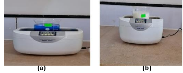
Figure. 2 The process of nano-fluids preparation, (a) CuO/H 2 O and (b) TiO 2 /H 2 O.
