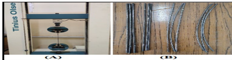
Figure 1: (A) Tensile test device (Tinnitus Olsen device)(B) Tensile test spacemen
