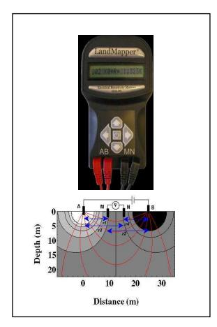
Fig. 4: Schema of current distribution in the soil by the LandMapper ERM-02 four-electrode probe(from http:// Landviser.net/web\_send/10, 2013).
