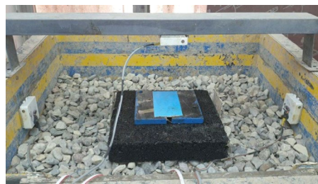
Figure 6: Pavement layers at unreinforced sample
