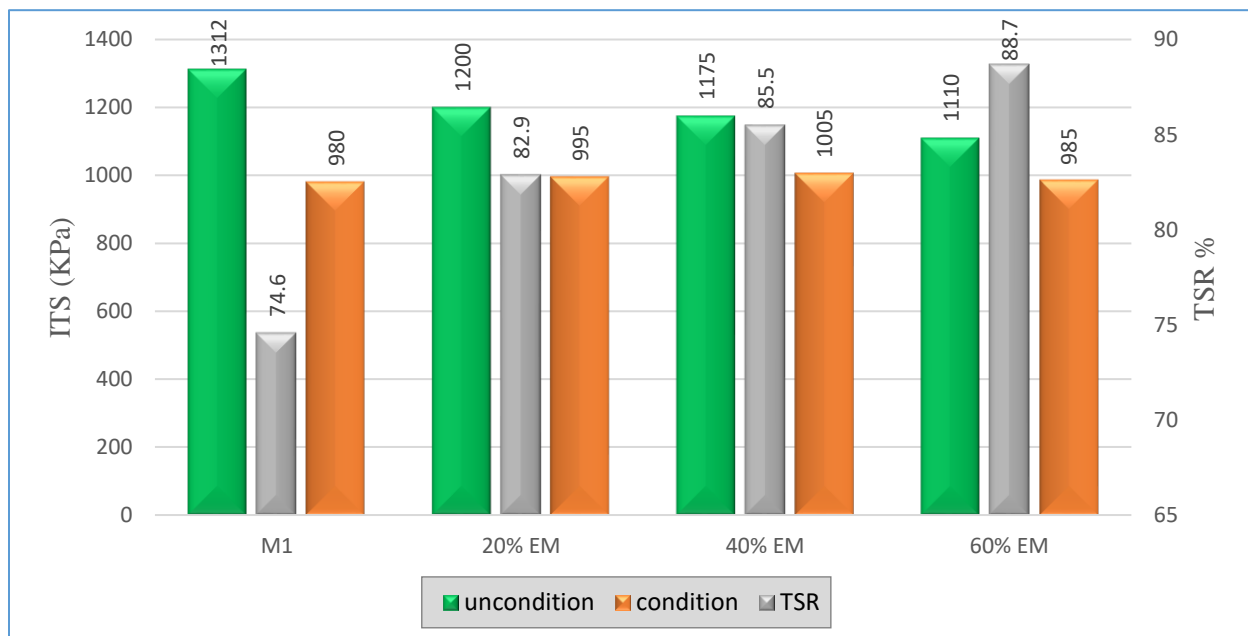
Figure 8 Tensile Strength Ratio (TSR) for various mixtures
