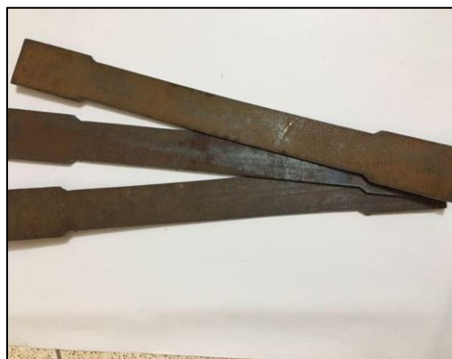
Plate (1) Typical tensile test of coupons
