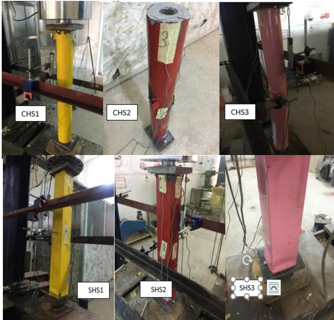
Plate (6) Mode failure of column
