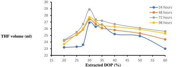
Figure 2. THF volume and extracted DOP at different temperatures for PVC plastic products after manufacturing.
