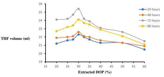
Figure 1. THF volume and extracted DOP at different temperatures for PVC plastic products before manufacturing.
