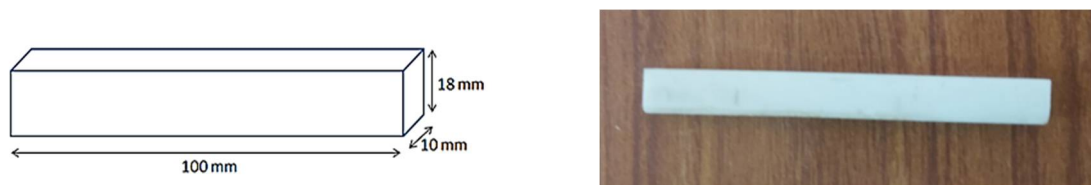
Figure 3: (A) (Schematic for Standard Flexural Test Specimen) , (B) ( Experimental Flexural Test Specimen before Testing
