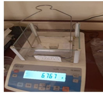
Figure 6: Measuring the piece's mass
