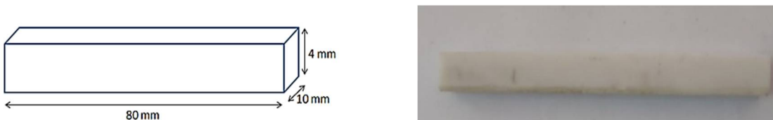
Figure 4: (A) Schematic for Standard Impact Test Specimen, (B) Impact Test Specimen
