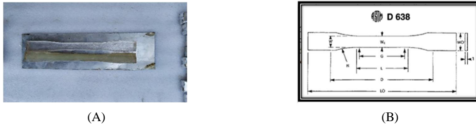
Figure 1: (A) Tensile test specimens mold (B) Standard geometry of ASTM (D 638)
