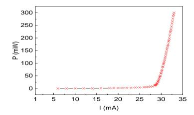
Fig. 1: I-P characteristics for the laser diode.
