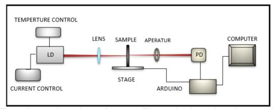
Fig. 3: Shows the experimental setup for z-scan. The rotational stage is used to move the sample on the axis.
