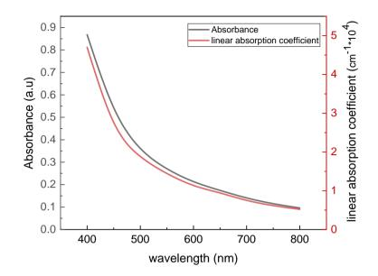
Fig. 2: Illustrated the absorption spectra and the linear absorption coefficient of ZnO thin films.
