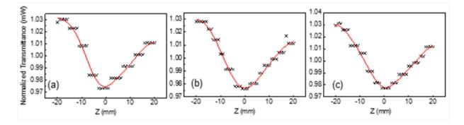
Fig. 4: Illustrates the normalized transmittance curves at open-aperture z-scan for ZnO thin films at different powers. (a) P = 1.9 mW; (b) P = 2.2 mW; (c) P = 2.5 mW.
