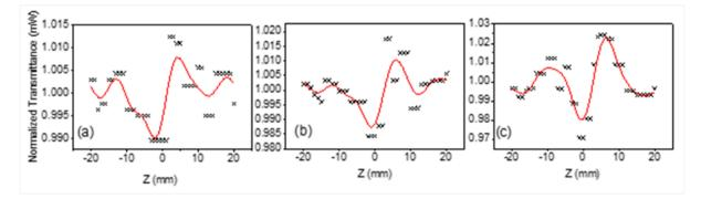
Fig. 5: Illustrates the normalized transmittance curves at closed-aperture z-scan for ZnO thin films at different powers. (a) P = 1.9 mW; (b) P = 2.2 mW; (c) P = 2.5 mW.
